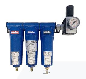
Compressed air filters, for wall mounting, are available for processing compressed air from an operational compressed air network into clean breathing air. In this way, users are permanently and safely supplied with breathing air. In the standard version, the wall-mounted unit, with an air flow rate of 500 l/min (30 m³/h), supplies max. two persons wearing breathing apparatus.
